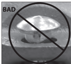
OVAL NECK OF BOLT NOT SEATED PROPERLY
