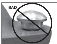
OVAL NECK OF BOLT NOT SEATED PROPERLY
