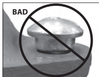
OVAL NECK OF BOLT NOT SEATED PROPERLY
