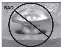
OVAL NECK OF BOLT NOT SEATED PROPERLY
