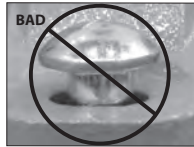
OVAL NECK OF BOLT NOT SEATED PROPERLY
