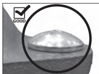
OVAL NECK OF BOLT SEATED PROPERLY
