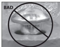
OVAL NECK OF BOLT NOT SEATED PROPERLY
