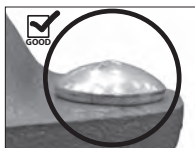
OVAL NECK OF BOLT SEATED PROPERLY
