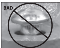
OVAL NECK OF BOLT NOT SEATED PROPERLY
