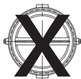
Incorrect Orientation for Horizontal Installation
