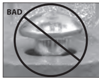
OVAL NECK OF BOLT NOT SEATED PROPERLY
