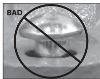
OVAL NECK OF BOLT NOT SEATED PROPERLY
