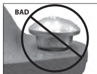
OVAL NECK OF BOLT NOT SEATED PROPERLY
