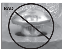
OVAL NECK OF BOLT NOT SEATED PROPERLY
