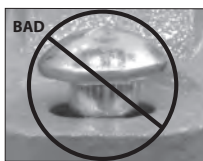
OVAL NECK OF BOLT NOT SEATED PROPERLY
