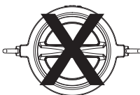
Incorrect Orientation for Horizontal Installation
