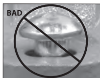
OVAL NECK OF BOLT NOT SEATED PROPERLY
