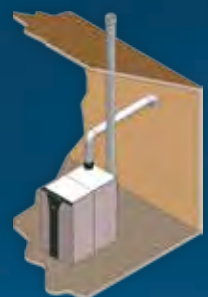
Vertical w/Sidewall Air
