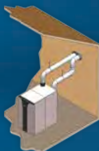
Direct Vent Sidewall
