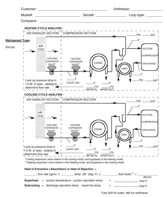
Note: Never connect refrigerant gauges during startup procedures. Conduct water-side analysis using P/T ports to determine water flow and temperature difference. If water-side analysis shows poor performance, refrigerant troubleshooting may be required. Connect refrigerant gauges as a last resort.
