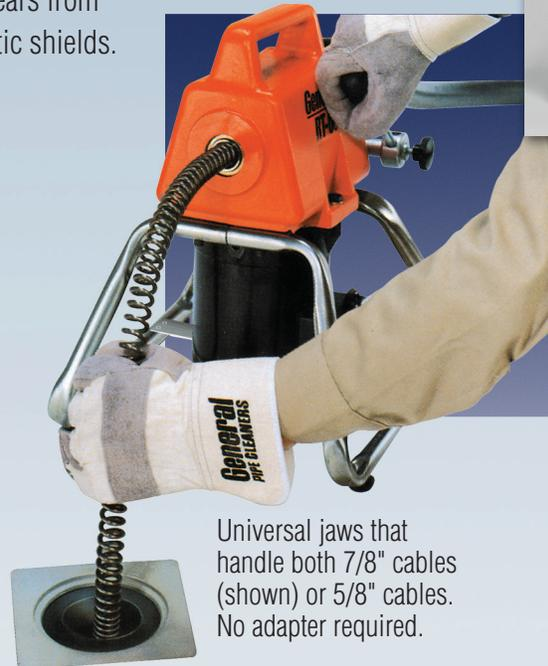
Universal jaws that handle both 7/8" cables (shown) or 5/8" cables. No adapter required.
