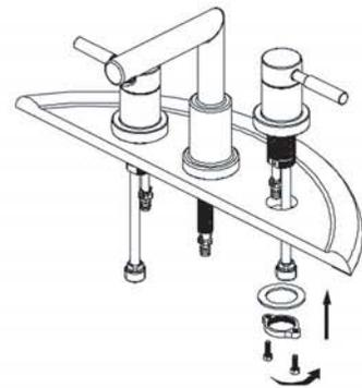
**3** Align tabs (1) and (2) on quick connects (3). Push quick connect housing firmly upward and snap onto receiving tube tab. Pull down moderately to ensure connection has been made. If it is necessary to remove quick connect, squeeze tabs on hose between index finger and thumb, then pull down to disconnect.
