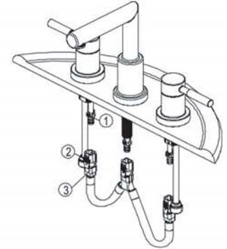
**4** Make connections to water lines. Use 1/2" IPS faucet connections (1) or use the supplied coupling nuts (3) with 3/8" O.D. ball nose risers (2). Use wrenches to tighten connections. Do not overtighten.
