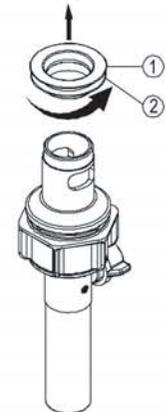
**6** Add Teflon Tape (1) to the drain body (2). Apply the provided gasket or plumber's putty to the underside of the flange (3). Insert the threaded end of the drain body up through the drain hole and attach flange to the body with the pivot (4) pointing to the rear of the sink.
