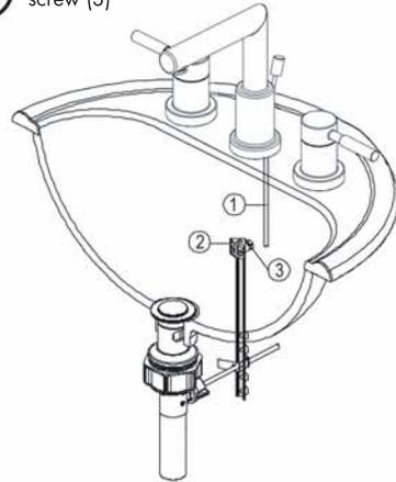
**8** Tighten nut (1) clockwise until the pop-up drain assembly is secure.
