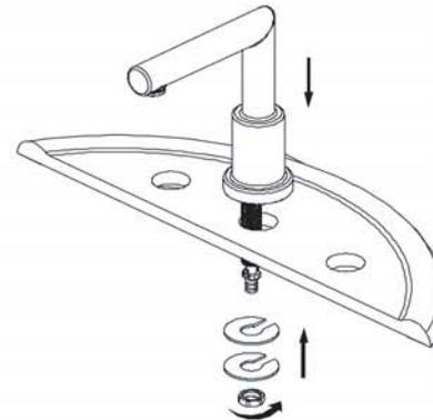
**2** Slide Hot and Cold end valves thru sink mounting holes. Make sure long tubes are installed facing away from spout. **Note: Hot side end valve is labeled.** Secure end valves with washers and nuts. Hand tighten nuts onto shank. Lock nuts into position by tightening screws.
