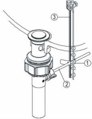
**7** Unscrew the nut (1) from the pop-up body. Note: retain the seal (2) on the horizontal rod (3). Place the nut onto the horizontal rod and insert the rod and seal (2) into the pivot hole (4). Install stopper (5) as non removable (6). Slide nut (1) on and hand tighten only.
