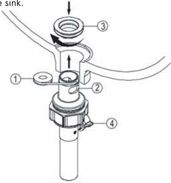
**9** Place one end of spring clip (1) on the end of horizontal rod (2). Insert rod through hole in lift rod strap (3). Secure with spring clip (1).
