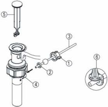
**10** Insert lift rod (1) into strap (2) and tighten screw (3)
