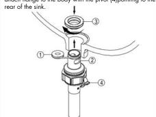
Unscrew the nut (1) from the pop-up body. Note: retain the seal (2) on the horizontal rod (3). Place the nut onto the horizontal rod and insert the rod and seal (2) into the pivot hole (4). Install stopper (5) as non removable (6). Slide nut (1) on and hand tighten only
