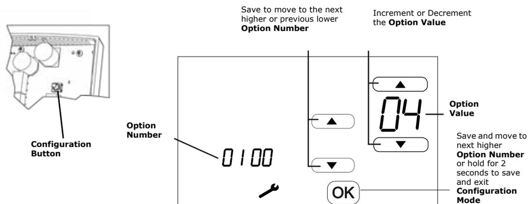
**Note:** Configuration mode automatically ends if no buttons are pressed for 10 minutes.
