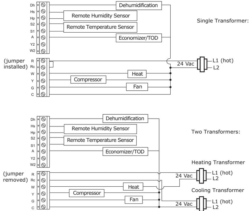
**Figure 5. Programmable Thermostat, 1H/1C, Heat Pump Without Auxiliary Heat (Option 2)**
