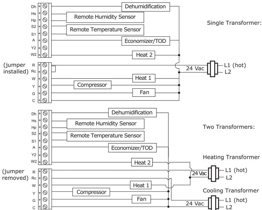
Figure 12. Programmable Thermostat, 1H/2C, Conventional (Option 9)
