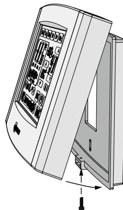
Install security screw to deter tampering.
