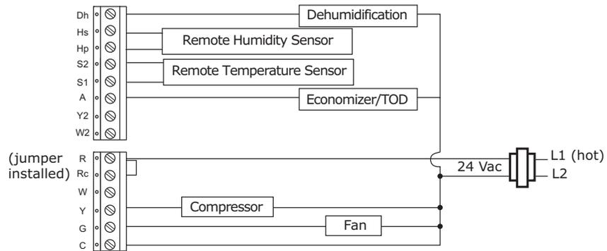
**Figure 9. Programmable Thermostat, 2H/1C, Heat Pump With Auxiliary Heat (Option 6)**
