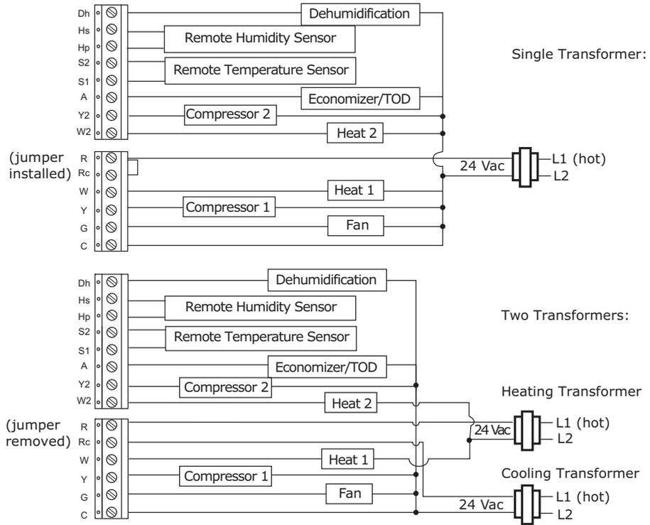
Figure 11. Programmable Thermostat, 2H/1C, Conventional (Option 8)
