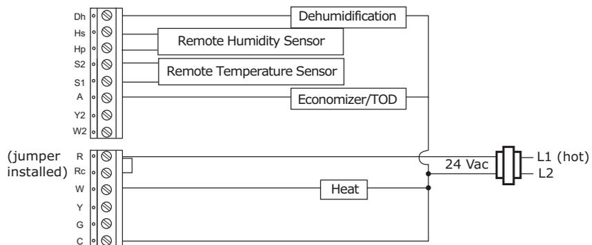
**Figure 7. Programmable Thermostat, 1H, Conventional With Fan (Option 4)**
