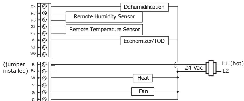
**Figure 8. Programmable Thermostat, 1C, Conventional (Option 5)**
