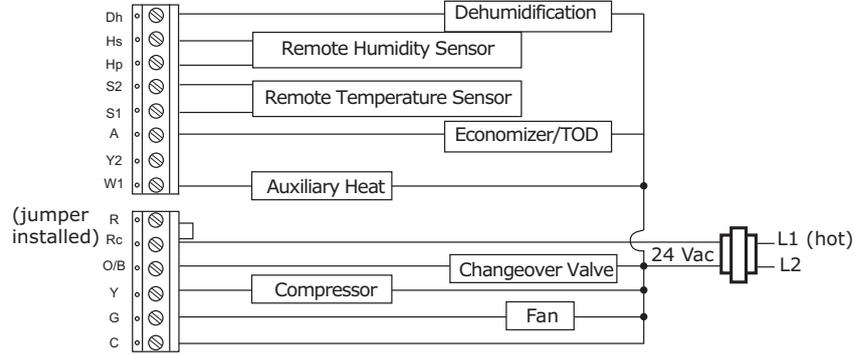
**Figure 10. Programmable Thermostat, 2H/2C, Conventional (Option 7)**
