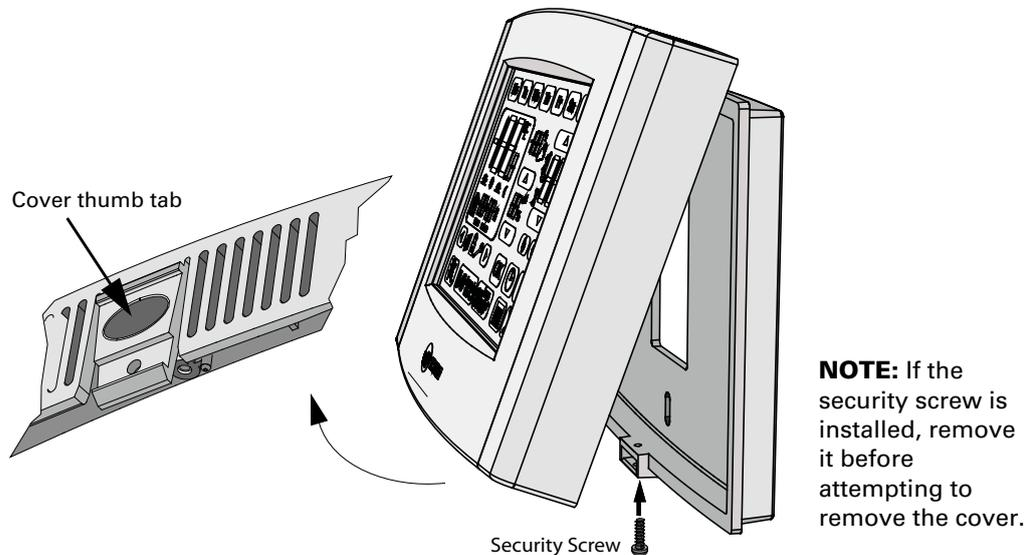
2. Push the cover thumb tab to release the cover from the backplate as shown above.
