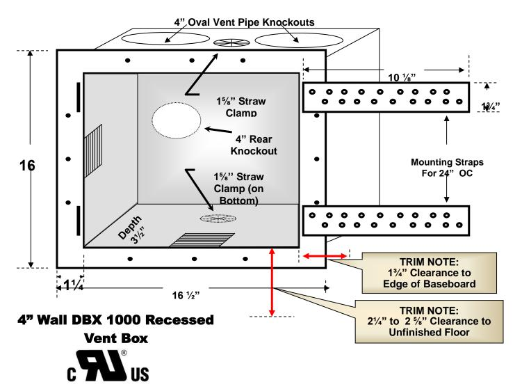
Made of High Impact Polystyrene Which Meets UL Standards for 94HB Flammability Testing and is recognized by Underwriters Laboratories Inc. Representative samples of this component have been evaluated by UL and meet applicable UL requirements. Provide a 16" or 24" on center stud bay with  $2 \times 6$  or  $2 \times 4$  wall structure.
