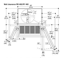
The drawing is based on a cabinet panel width of  $^3/_4{}^{\rm H}$  (19 mm) and a Gaggenau cabinet handle height of  $1^5/_1{\rm e}^*$  (49 mm).
