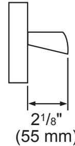
\*Protrusion of handle from outer part of door. Does not include thickness of door
