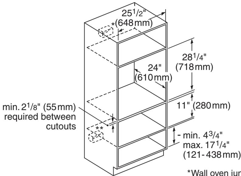
\* Wall oven junction box may be located above or right or left of the unit within reach of the power conduit.
