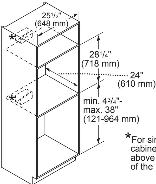
\* For single ovens installed into a wall cabinet, the junction box may be located above or beneath the unit within reach of the power cord.
