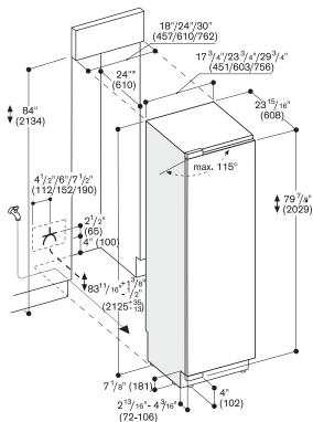
The door face dimensions are designed for a maximum gap of 1/8" (3 mm). \* For a flush-mounted appearance, the minimum cut-out depth must be 25". See
