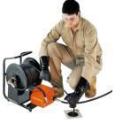
The Foot Pedal interrupts the flow of water between the pump and the nozzle while leaving both hands free to guide the hose. Position the Handy-Reel at the drain site. Connect the jet machine to the inlet on the Foot Pedal. Select and attach nozzle to the hose on the reel. Put the hose 2 to 3 ft. into the drain line. Follow the start-up procedures.
