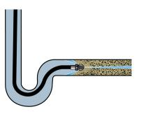
notice less vibration with a 1/4" hose, and almost none with a 3/8" hose. However, the pulse is still effective, causing the water to burst from the nozzle hundreds of times per second. If you are still having difficulty getting hose around a tight bend, switch to a smaller diameter hose. Turn the pulse off before turning machine off.
