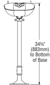
All dimensions assume standard thread engagement. Variations in manufacturing allow for +/- 1/8" (3mm) per threaded joint. To find the tolerance of a dimension, add the number of thread joints across the length of the dimension and multiply it by 1/8" (3mm).
