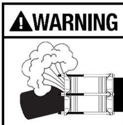
**THIS PRODUCT DOES NOT RESTRAIN PIPE MOVEMENT. Proper anchoring is required to prevent pipe pull out. Failure to anchor or improper anchoring can result in dangerous pipe content escape, property damage, serious injury, and/or death. Read the product installation instructions prior to installing this product.**
