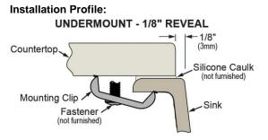
Designed to affix to the underside of any solid surface countertop.
