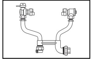
**ANGLE BALL VALVE BY ANGLE CHECK VALVE (1" METER)**
