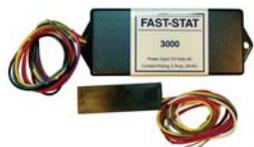
Model 3000 provides 4-wire control over 2-wire cable or 6-wire control over a 4-wire cable. With a 2-wire cable it can provide “R”, “W”, “G” and “Y”. With a 4-wire cable it can provide “R”, “W”, “Y”, “G”, plus any two of “C”, “D”, “W2”, “Y2” or “O/B”. Common uses include adding air conditioning to a heating system. Can also be used for heat pumps, 2-stage heating or cooling when an existing 4-wire thermostat cable is present.
