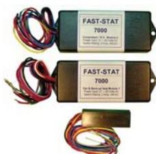
Model 7000 provides 7-wire control from the thermostat to the furnace or fan-coil over a 4-wire cable. This includes “R”, “C”, “G”, “W”, “Y1”, “Y2” and “O/B”. From the furnace or fan-coil to the heat pump it provides 6-wire control over a 2-wire cable. This includes “R”, “C”, “Y1”, “Y2”, “O/B” and “W” (defrost). Common uses include converting from an air conditioning to a heat pump (single or 2-stage) system.
