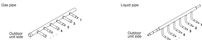
4. Install the supplied closed pipes to the header outlets that will remain unused.
