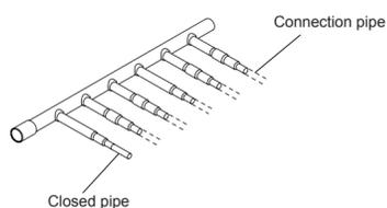
5. Place the Header horizontally so that the refrigerant separates evenly. They cannot be used vertically.
