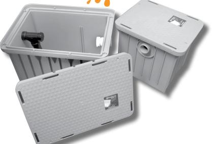
Installed on a wide range of applications, where by gravity, fine material is required to be separated from the waste water flow. This includes materials such as plaster, clay, sand, sediment, grit and general debris. Any material heavier than water can be successfully separated in the Endura Plaster Trap.
