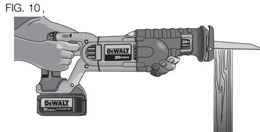
**⚠WARNING:** Use extra caution when cutting overhead and pay particular attention to overhead wires which may be hidden from view. Anticipate the path of falling branches and debris ahead of time.
