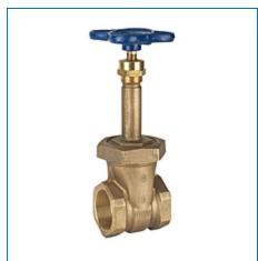
**Specifications UPC** Code 039923618313 Gate Valve Type **Valve Size** 1/2 in Material **BRZ Cast Bronze** Description T134 1/2 THD 150# RS GATE BRZ Multi-Turn **Turns / Operation** Seat / Seal Material **Bronze Connection Type** T -- Female NPT Thread (FIPT) Valve Gate Stem Design RS - Rising Stem Valve Multi-Turn Bonnet Design Union Bonnet Standard Handwheel **Operation Type**
