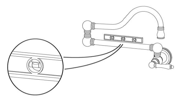
9. Tighten the two set screws onto the injector until fastened. Then, push back escutcheon up to finished wall.
