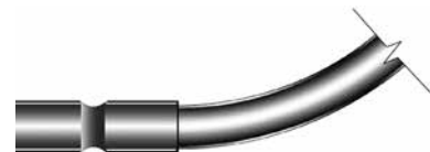
Deep Socket PVC Coupling bonded onto fiberglass elbow.
