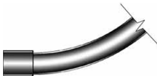
Standard PVC Coupling bonded onto fiberglass elbow.
