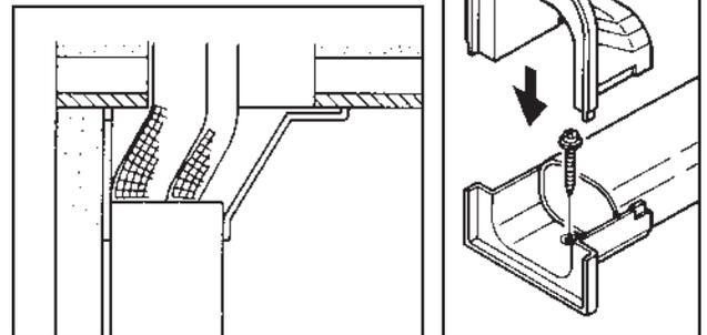
Detail of SP Soffit Inlet
