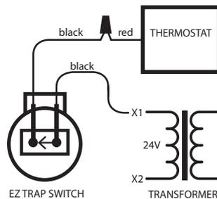
**Note:** Wiring diagram shown cuts power to thermostat when float switch operates to stop operation of the A/C unit. To inhibit mold growth during long absences, connect terminals into yellow cooling circuit so when float switch operates, condenser will switch off but fan will continue running.
