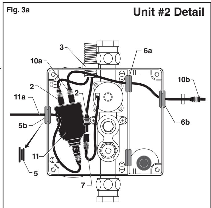
**CAUTION:** Use only American Standard supplied cable sets. Using non-AS supplied cables, or cutting, splicing or modifying any components will void the warranty.
