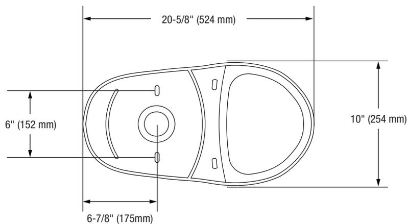
Note: All dimensions and specifications are nominal and may vary: Dimensions of 8" and greater have a tolerances of +3%. Dimensions less than 8" have a tolerances of +5%.
