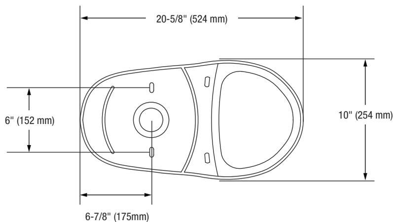
Note: All dimensions and specifications are nominal and may vary: Dimensions of 8" and greater have a tolerances of +3%. Dimensions less than 8" have a tolerances of +5%.
