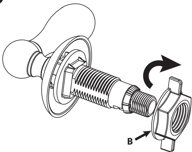
Unscrew the tank nut (B). The thread for the tank nut is a left handed thread.
