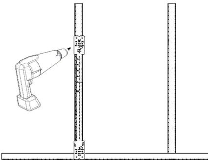
Set to desired height for box  $\mathcal{C}$ . Align on stud. Attach screw through keyhole.
