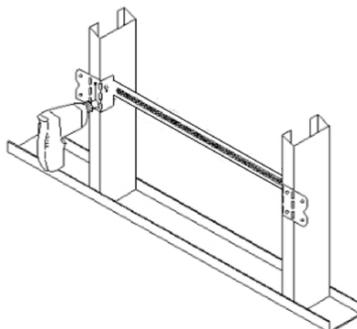
Use screw gun to assemble to stud.
