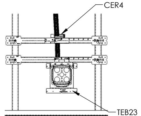
May be used with CER4 as cable support. Attach TEB23 box mount at desired location.
