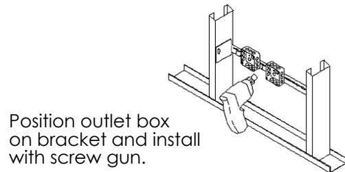
Position outlet box on bracket and install with screw gun.
