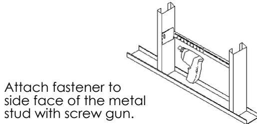
Attach fastener to side face of the metal stud with screw gun.
