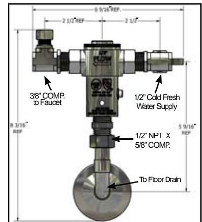
The Priming valve must have a min. elevation of 12" (305mm) above the finished floor.
