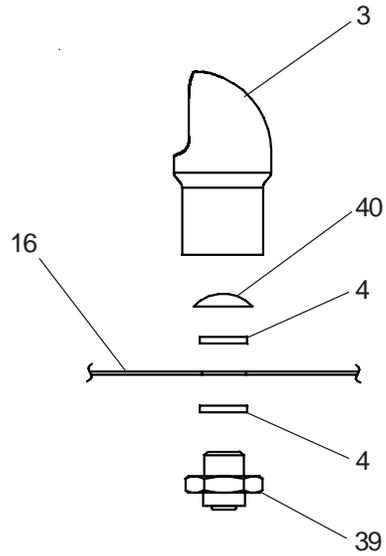
Fig. 26- Smart Flow™ Bubbler Detail
