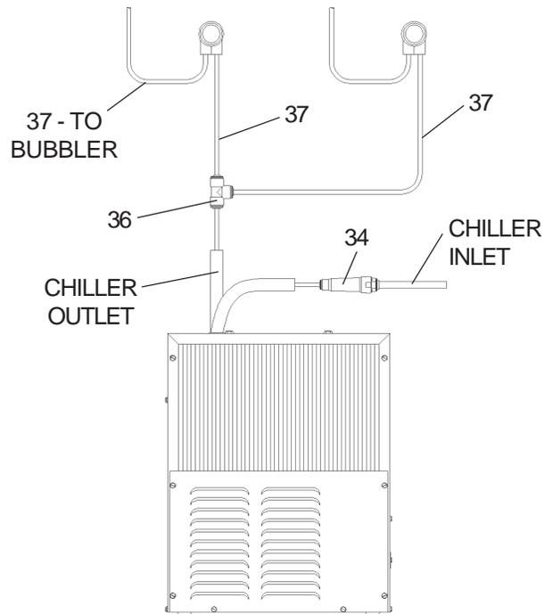
Figure 18 – OVL-II SER-Q/ESR-Q Tube Routing
