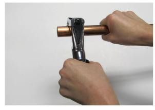
1. Make a clean cut onto the copper, CPVC, or PEX tubing. Deburr the edges to ensure that the outside diameter is free of sharp ridges.
