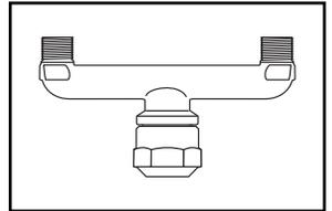
QUICK JOINT FOR COPPER OR PLASTIC TUBING (CTS) INLET BY TWO MALE IRON PIPE THREAD OUTLETS
