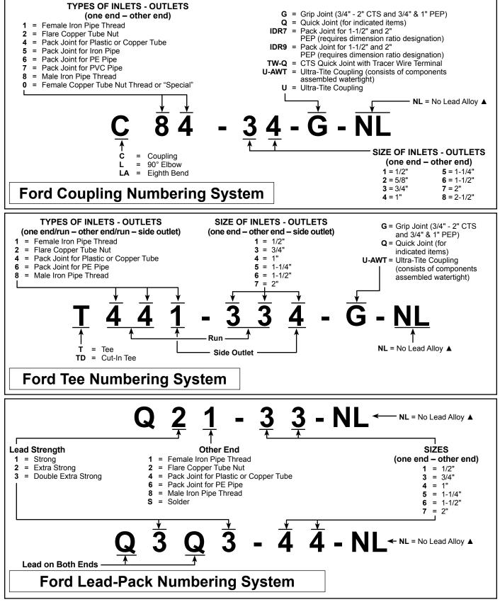
▲ Ford Meter Box no-lead brass products manufactured from UNS/CDA No. 89833 alloy shall contain no more than 0.25% total lead content by weight.
