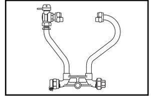
ANGLE BALL VALVE BY METER NUT (5/8" X 3/4" METER)
