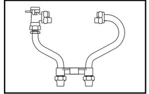
ANGLE KEY VALVE BY METER NUT (5/8" x 3/4" METER)
