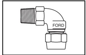
**MALE IRON PIPE THREAD BY GRIP JOINT FOR POLYETHYLENE PIPE (SIDR7 PEP)**
