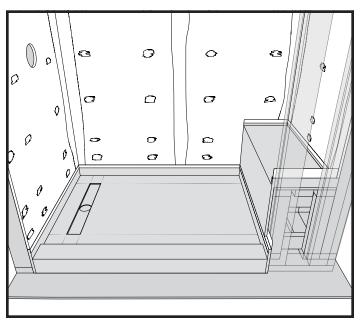
6. Install the shower backer board and waterproofing in accordance with the standards established by the Tile Council of North America, Inc. Seal and waterproof joint between backer board and the shower pan splash walls using Redi Flash or 100% silicone. It is recommended to use a membrane and fluid applied waterproof in addition to the Redi Flash or 100% silicone.
