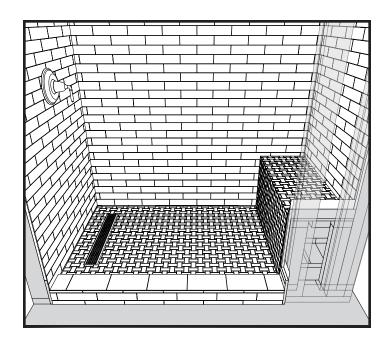
7. Adjust the height of the drain as necessary to accommodate the floor covering. Set your tile using a white modified thin-set/tile mortar and a notched trowel as specified by the thin-set/tile mortar manufacturer based on your tile size. Tile Redi recommends the modified thin-set/tile mortar products found in table below.
