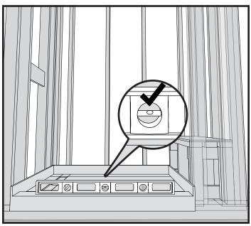
2. Install your Tile Redi shower pan according to the instructions. Using a level, ensure that the pan is level left to right, and front to back along the splash walls. Also make sure the pan is level left to right along the curb.
