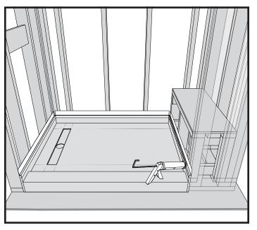
3. Install the Redi Flash flashing system along the splash walls of the shower pan. Apply a bead of 100% silicone to the top of the Redi Flash flashing that runs along the splash wall alongside the bench frame.
