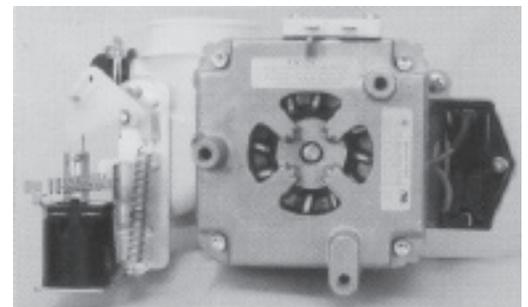
Note - On Electronic Drain Feedback switch models, install the adapter bracket (11) to the solenoid using the 2 screws
