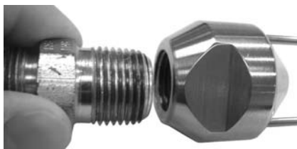
Figure 4 – Installing Adapter Into Cone
