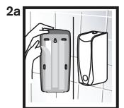
Use the alcohol wipe provided to thoroughly clean any surface that will have adhesive tape attached. Pull off the protective backing off the adhesive tape and mount the dispenser to the wall holding it in place for 10-15 seconds allowing the tape to adhere to the mounting surface. Remove the batteries from the dispenser. Let the dispenser set up for 24 hours before installing the batteries and refill.
