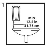
The dispenser should be mounted 12.5 inches (31.75 cm) above the counter-top, sink or other surface. If an object remains in the sensing range for more then 10 seconds, the green LED will flash and no soap will be dispensed after the initial dose. Remove object and unit will operate normally
