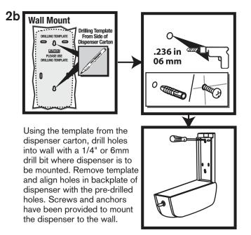
NOTE: Insure that proper mounting hardware is used for your particular wall composition.
