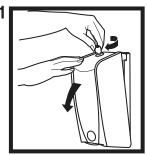
Use the dispenser cabinet key to open the front cover. Insert the key into the holes located at the top of the dispenser, twisting the key, and pulling the cover towards you. The cover is hinged at the bottom of the dispenser.
