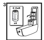
Insert four C-cell **alkaline** batteries (not included) making sure to place batteries in the compartment in the proper orientation as shown by the diagram in the battery compartment.
