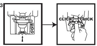
Snap the pouch fitment into the U-shaped bracket insuring the nozzle fits into actuator lever. The pouch fitment will snap into place once both brackets have snapped over the fitment.
