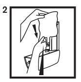
Remove the refill pouch from the packaging box. Place the refill pouch with the nozzle pointing down into the pouch holder. Remove and discard the nozzle cap.
