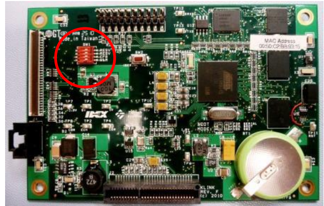
Figure 6.5 CPU DIP Switches for Program and W&M Access (rev 2.x)
