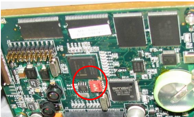
Figure 6.4 CPU DIP Switches for Program and W&M Access (rev 1.0)
