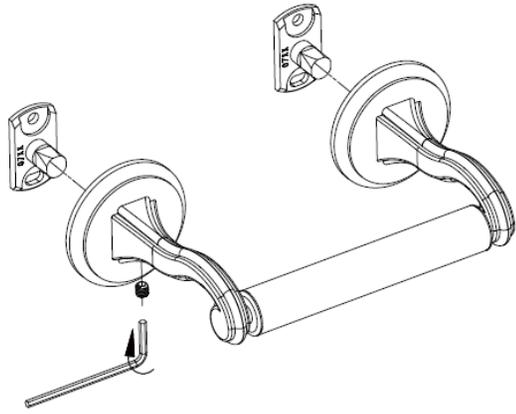
② ALIGN MOUNTING BRACKETS AND MARK LOCATION
