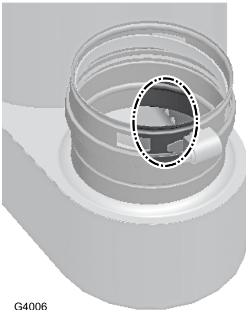
Figure 83 Recuperator flue way drain holes
