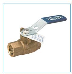
**Specifications UPC** Code 039923681409 Ball Valve Type **Connection Type** T -- Female NPT Thread (FIPT) Valve Size 3/4 Seal Material RPTFE (Reinforced) **Seat Material** RPTFE (Reinforced) Stem Material SS - Stainless Steel **Ball Material** Stainless Steel **Body Material** Bronze CS Extended Lever Handle Valve Operator
