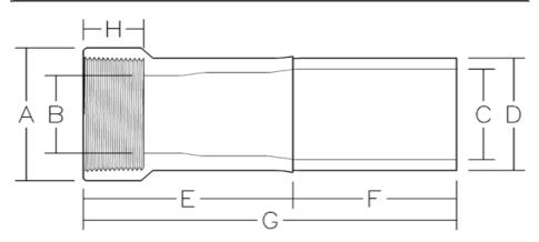
Fully pressure rated • Standard SDR sizes 7,9,11,17 • Metric sizing available Manufactured to D3035, D1599, D1598, ASTM D3350
