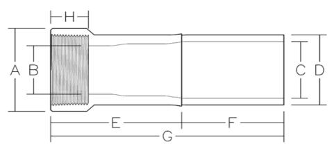
Fully pressure rated • Standard SDR sizes 7,9,11,17 • Metric sizing available Manufactured to D3035, D1599, D1598, ASTM D3350 11/00 ® Registered Trademark Poly-Cam, Inc. - US Patent # 5,211,429
