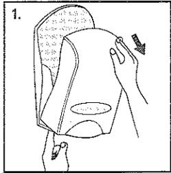
1. Open dispenser by pushing up on the release latch located at the bottom of the dispensers back plate. While pushing the release latch up, grasp dispenser cover with the other hand and pull downward.
