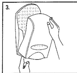
3. Open dispenser by pushing up on the release latch located at the bottom of the dispensers back plate. While pushing the release latch up, grasp dispenser cover with the other hand and pull downward.
