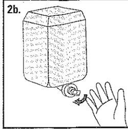
2b. For the liquid soap refill rotate the nozzle 1/4 turn so it points down.
