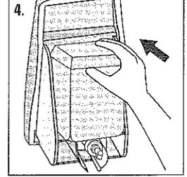
4. Lock the refill in place by sliding it into the slotted opening.
