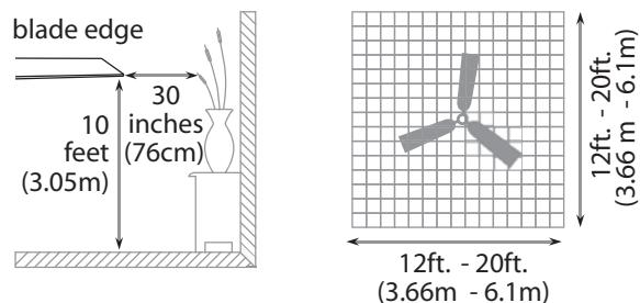
This fan can be mounted with a **downrod** on a normal ceiling **only**. Fan *cannot* mount as a flushmount installation *nor* on a vaulted ceiling.
