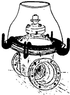
Gate Valve Adaptor installed on a valve with box.
