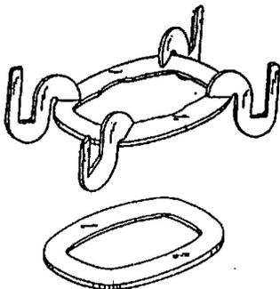
1/4" Steel with UV Polyurethane Protective Coating
