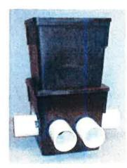
Our box riser is made of high density polyethylene and is easily assembled for installation. It can be provided as both gas and watertight. It also screws into the lower unit with s/s phillips head screws.
